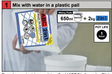
Pour clean water into a container & add ABC 2 in 1 powder. Stir to attain a lump-free, creamy consistency. Use immediately after mixing and strictly observe 1 hour pot life.
